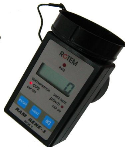
Fig. 2 Contamination reading Filter cup removed from detector and attached to the instrument
