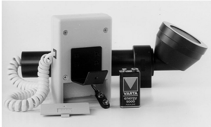
Figure 5-1. RAM SURF Battery Compartment
